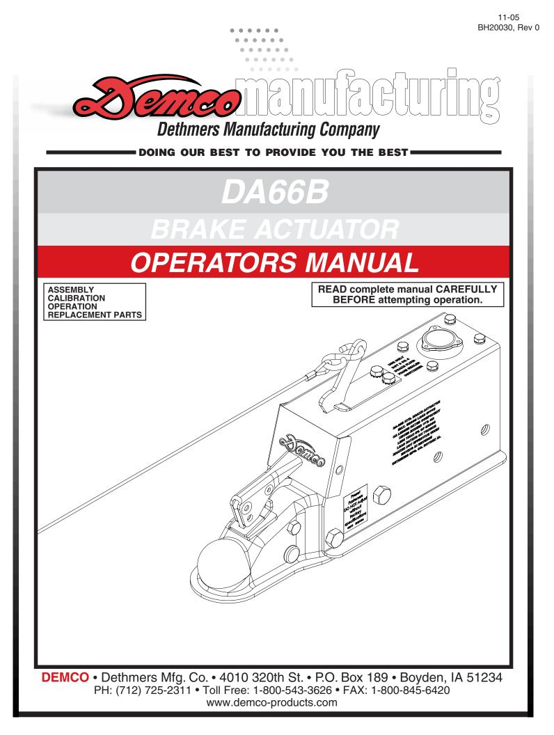
Model DA66B is a hydraulic surge brake actuator for trailers with two or four wheels. When brakes are applied on the towing vehicle, forward inertia of trailer toward towing vehicle applies brakes on trailer in direct relation to manner brakes are applied on towing vehicle. Brake towing vehicle hard and brakes on trailer are applied hard. Master cylinder push rod spring assembly protects system from hydraulic pressure overload.
